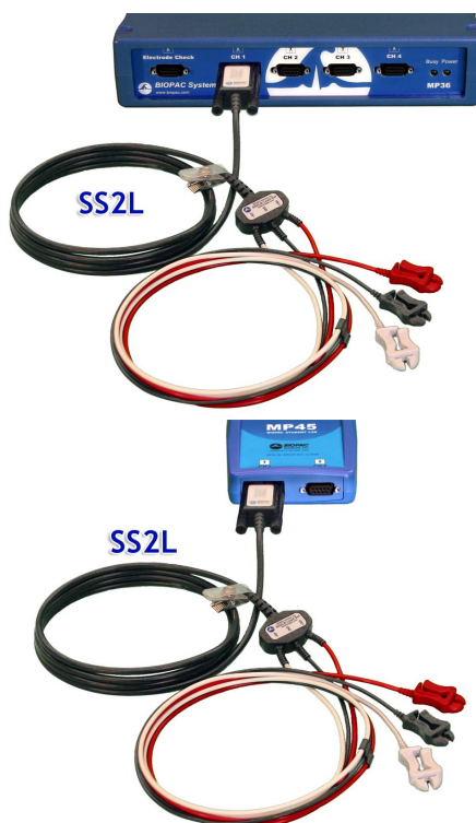
Fig. 4.2 MP3X (top) and MP45 (bottom) hardware connections
