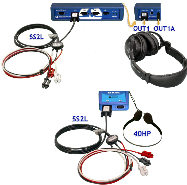
Fig. 1.4 MP3X (top) and MP45 (bottom) equipment connections
