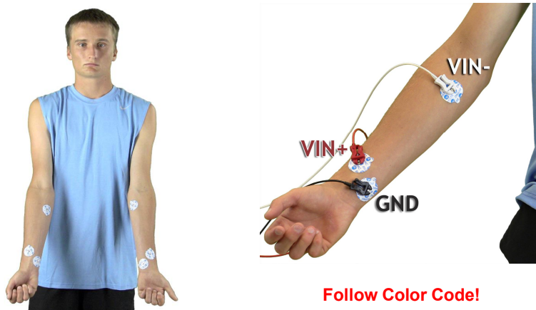
Fig. 1.5 Electrode placement and lead attachment
