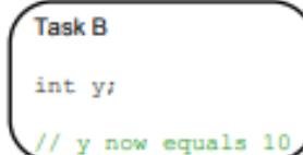
Task B has removed one item, leaving only the second value written by Task A remaining in the queue. This is the value Task B would receive next if it read from the queue again. The queue now has four empty spaces remaining.
