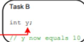
Task B reads (receives) from the queue into a different variable. The value received by Task B is the value from the head of the queue, which is the first value Task A wrote to the queue (10 in this illustration).
